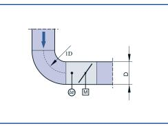
A radius bend with at least 1D radius at a centre line curvature – withou tan additional straight duct section up stream of the VAV terminal unit – has only a negligible effect on the volume flow rate accuracy. Junction
