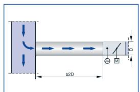
A junction causes strong turbulence. The stated volume flow rate accuracy  $\Delta V$  can only be achieved with a straight duct section of at least 2D length upstream. Shorter upstream sections require a perforated plate in the branch and before the VAV terminal unit. If there is no straight upstream section at all, the control will not be stable, even with a perforated plate.
